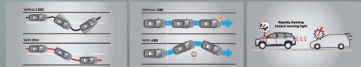
ESC (Electronic Stability Control), ABS (Anti-lock Braking System) EBD (Electronic Brake-force Distribution) BA (Brake Assist), ESS (Emergency Stop Signal)
