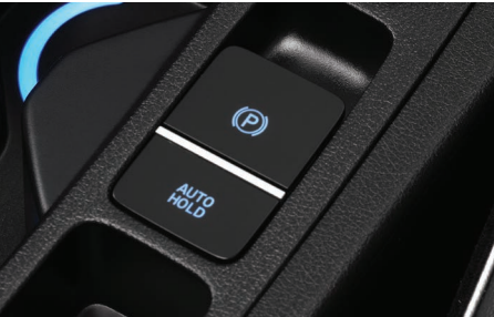
Electronic Parking Brake with Auto Hold
